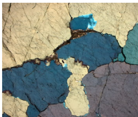
Crossed polar observation of rock thin sections
