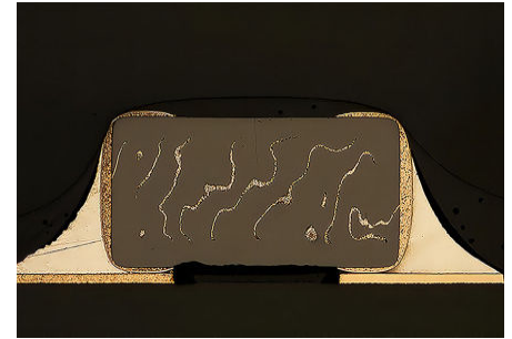
Capacitor tin plating height detection
