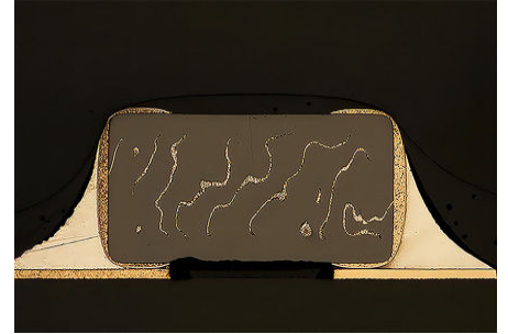
Capacitor tin plating height detection
