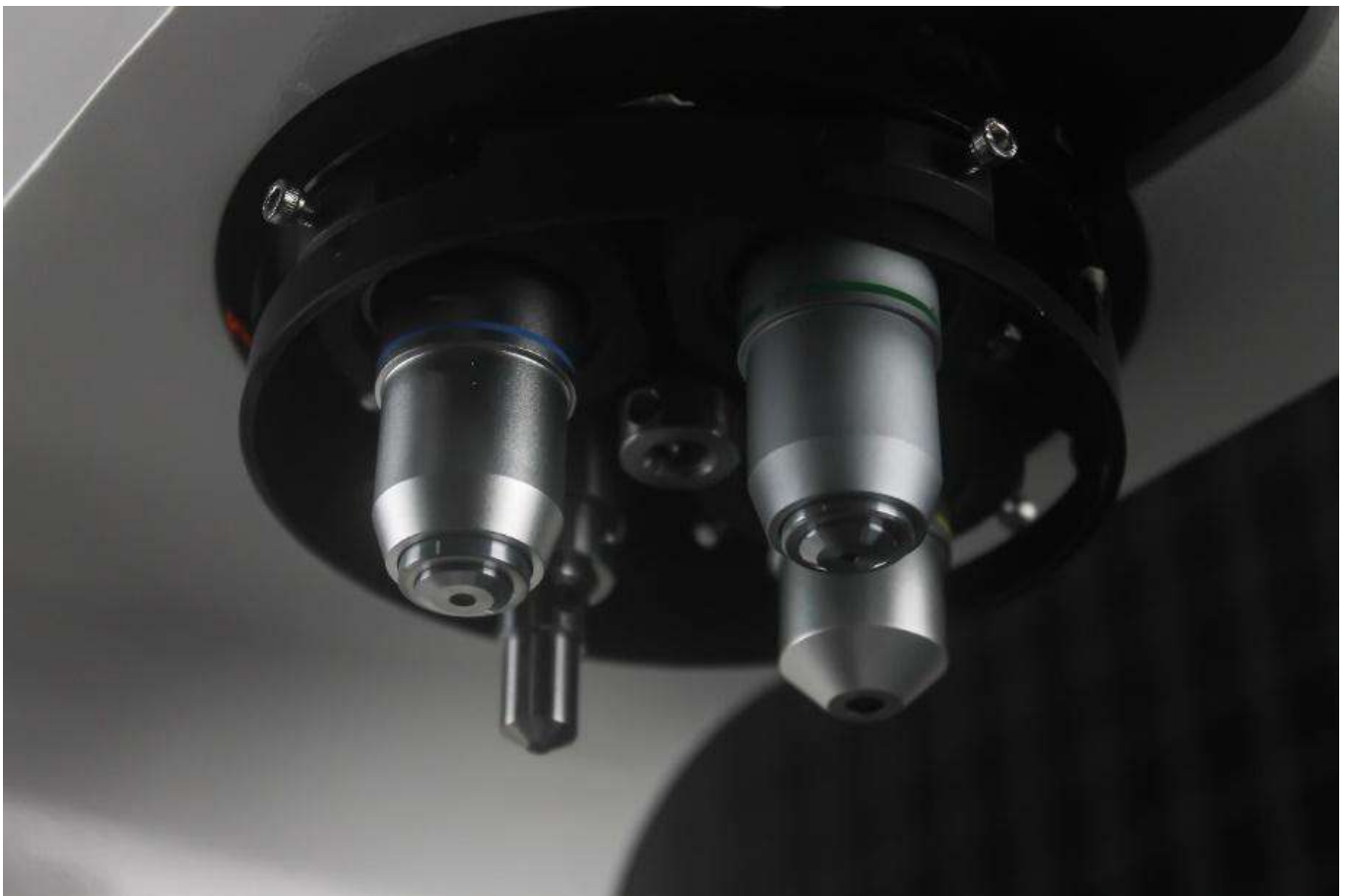
One Indentor with Three Objective Lens Realized
