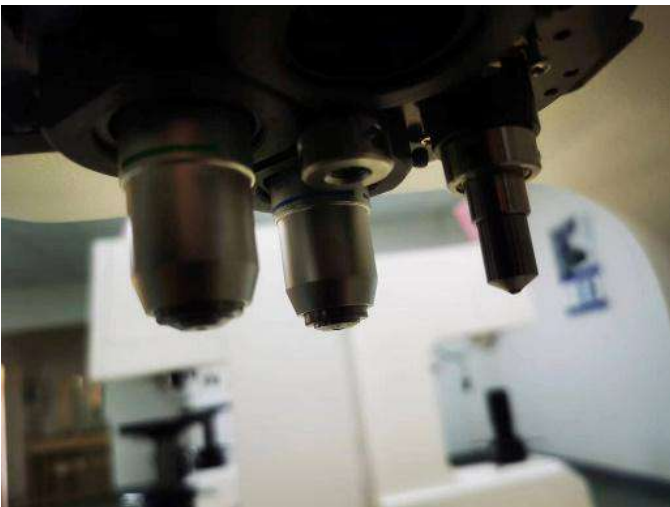
One Indenter with Two Objective System
