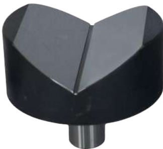
V-shaped Test Anvil
