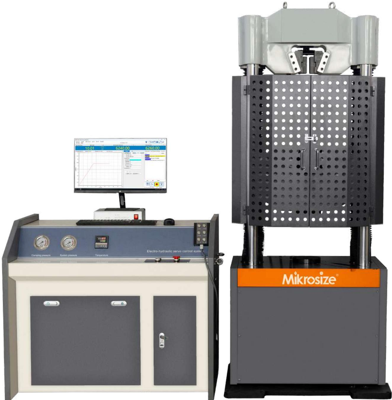
UTM-H300 Computerized Electro-Hydraulic Servo Hydraulic Universal Testing Machine
