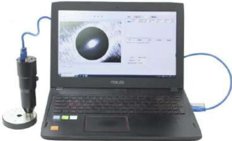
uVision-PB Portable Automatic Brinell Hardness Measurement System(without computer)
