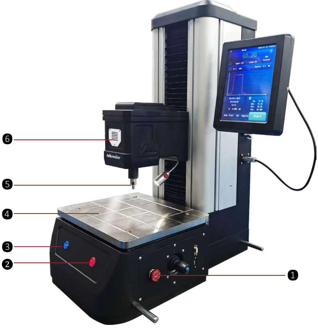
1. Emergency Stop Button 2. Stop Button 3. Start Button 4. Stage 5. Indenter 6. Downward Pressing Head
