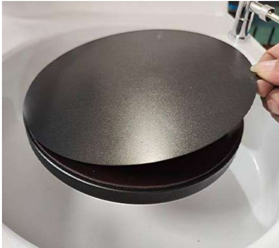
Put Teflon Pad on Magnetic Platen Disc
