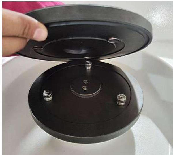
Magnetic Platen Disc Installation
