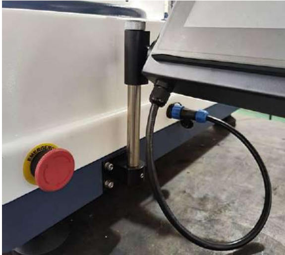
Connect Touch Screen to Aviation Plug
