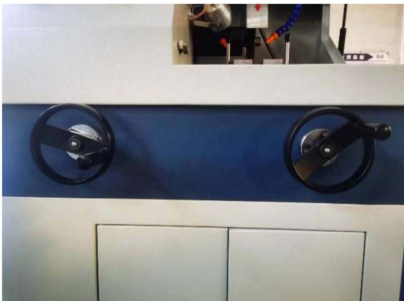
Z-axis Manual Adjusted by Rotating Handwheel(left)
