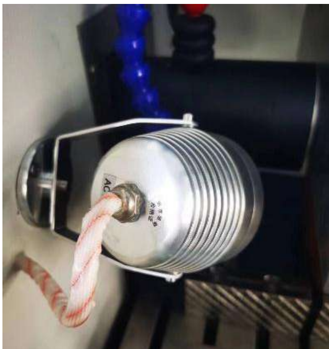
LED Illumination Inside Cutting Chamber
