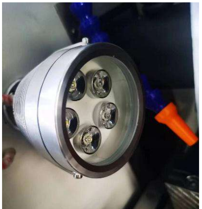
LED Illumination Inside Cutting Chamber
