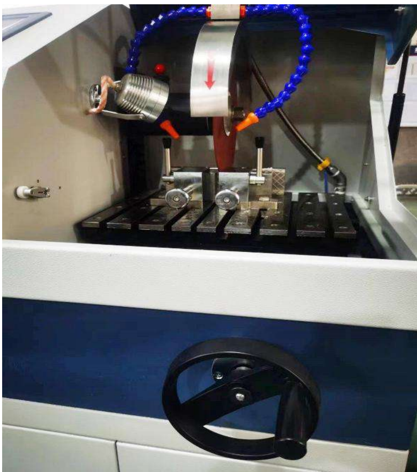
Y-axis Manual/Auto Adjusted by Rotating Handwheel
