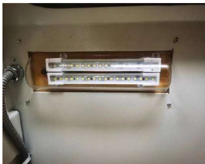
LED illumination inside Cutting Chamber
