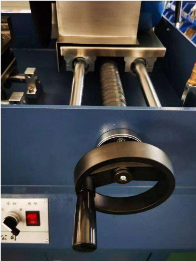
X-axis Controls Cutting
