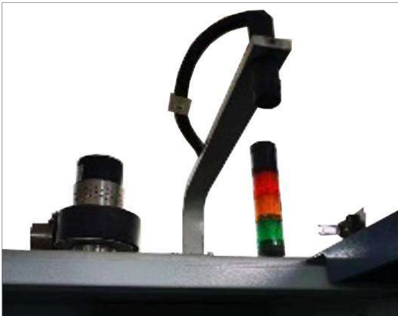
Gas Exhaust/ Laser Position /Signal Alarm Light
