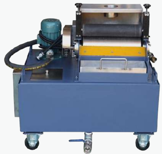
Magnetic Cooling Water Tank
