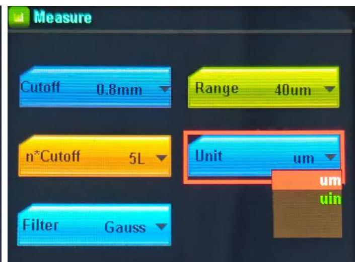
**The iSurfa-360 surface roughness tester offers a wide range of measurement conditions settings.**
