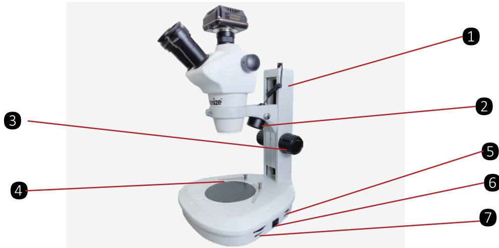
1.Mainframe 2.LED illumination 3.Focus knob 4.Fixed clamp 5.Epi-illumination knob 6. Switch 7.Transmitted illumination knob
