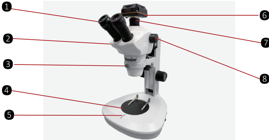
1.Eyepiece 2.Zoom lens tube 3.Screw for fasten zoom lens tube 4.Mechanical stage 5.Screw for fasten mechanical stage 6.CCD camera 7.Adapter 8.Zoom knob
