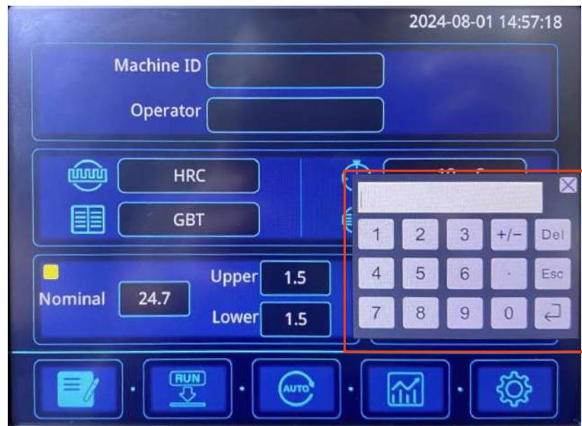
Users can choose the appropriate loading time, the default is 5 seconds, generally no need to adjust, the range is 2 ~ 60 seconds.
