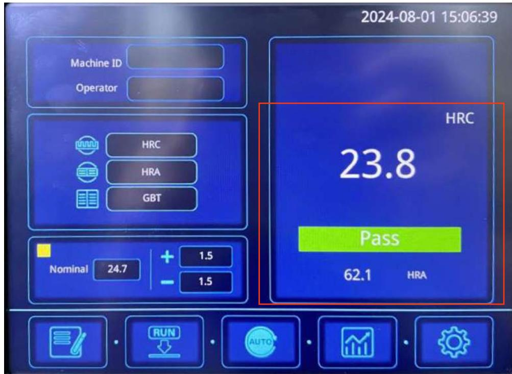
When the user finished measuring, you can view the results of this measurement in the display interface, if the measurement result is within the deviation, the interface will display "PASS", it will also display the measurement scale set by the user, the conversion scale, the standard and the standard value set by the user, and the upper and lower deviation.
