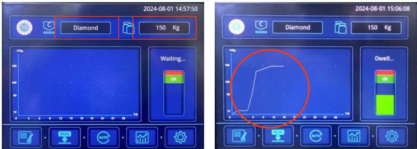
After the user selects the experimental scale, the test interface will automatically match the corresponding test force and the indenter to be selected.
