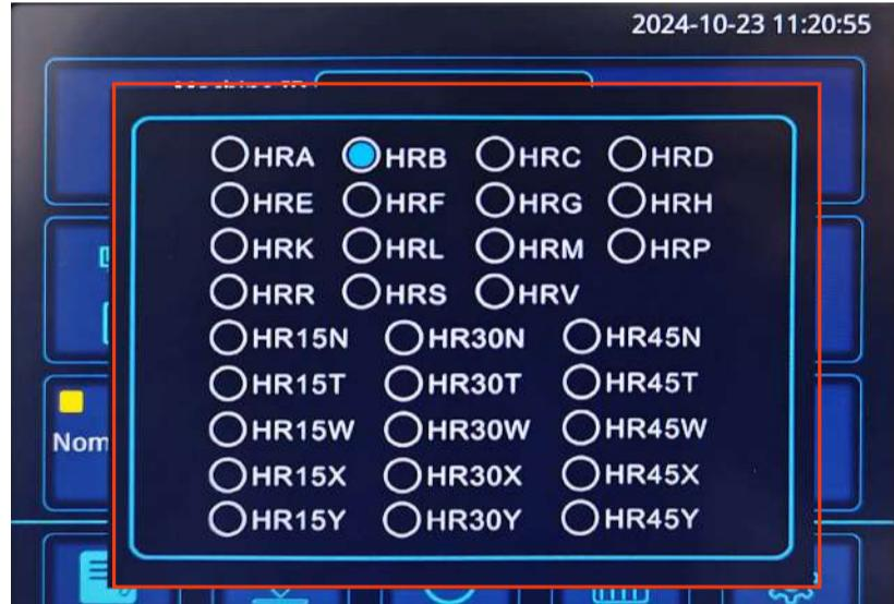
Hardness scales supported by the machine: HRA, HR-B, HRC, HRD, HRE, HRF, HRG, HRH, HK, HRL, HRM, HRP, HR-R, HRS, HRV, HR15N, HR30N, HR45N, HR15T, HR30T, HR45T, HR15W, HR30W, HR45W, HR15X, HR30X, HR45X, HR15Y, HR30Y, HR45Y
