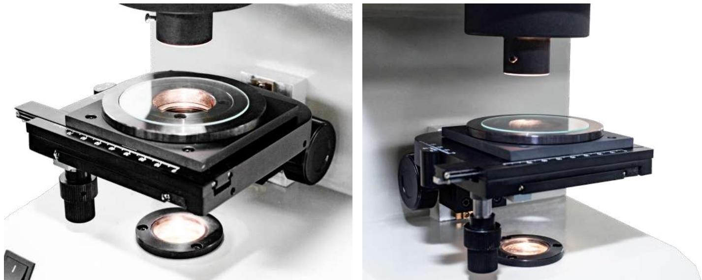
The workbench has strong adaptability. The square workbench measures 110×125mm and has a diameter of 90mm. It is equipped with a 70mm diameter transparent glass, which can stably support various J-specification impact test samples and meet the placement requirements for different specifications of samples. At the same time, the glass material ensures the light transmission of the light source, without affecting the detection imaging.
