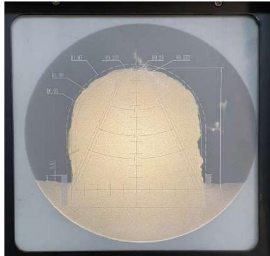
The size is highly adaptable. the 200×200mm specification can fully display the enlarged V/U-shaped notch outline without any field limitation, making it convenient for observing details.
