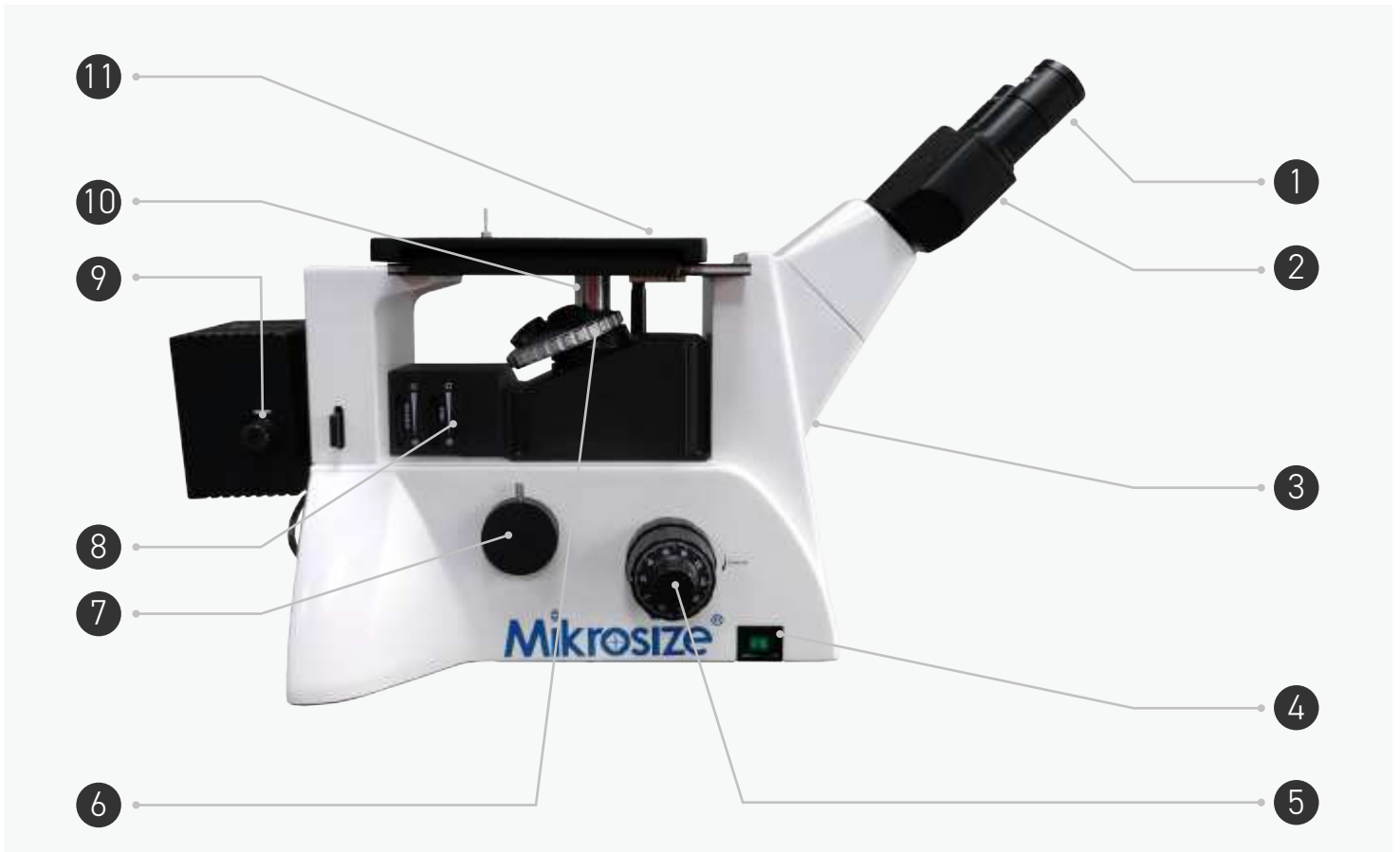
1.Eyepiece 2. Eyepiece tube 3. Main frame 4. Power switch 5. Coarse/fine focusing mechanism 6. Nosepiece 7. Camera device 8. Reflected illuminator 9. Lamp house 10. Objective 11. Stage
