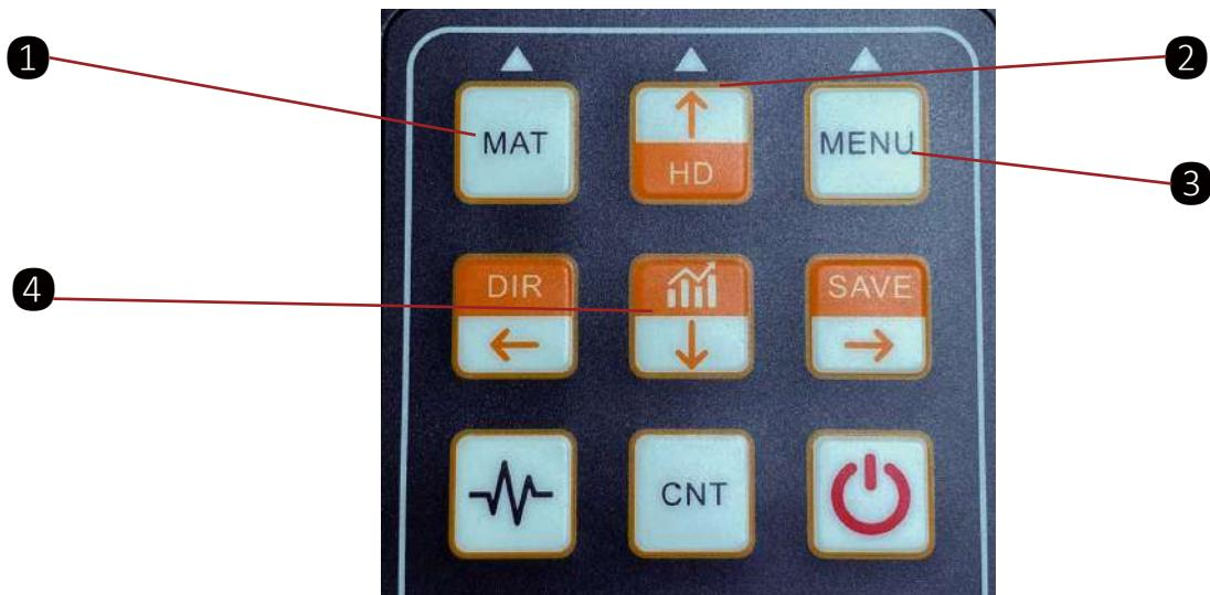
**1. Material Selection Key      2. Up Arrow Key / Hardness Scale Selection Key**
