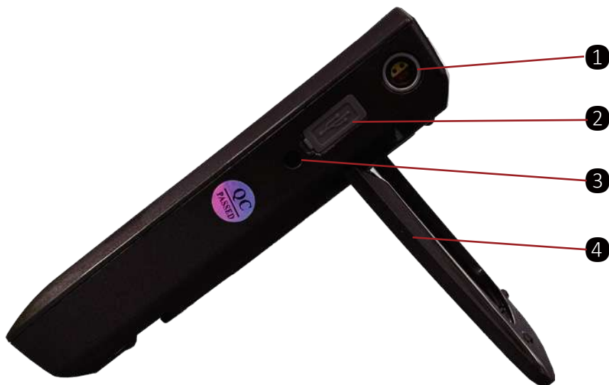
1. Sensor Jack 2. USB Jack 3. Charging Jack 4. Stand
