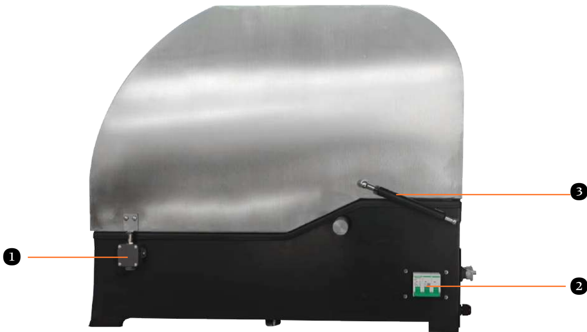
1. Closed-door Detection 2. Switch 3. Protective housing support rod
