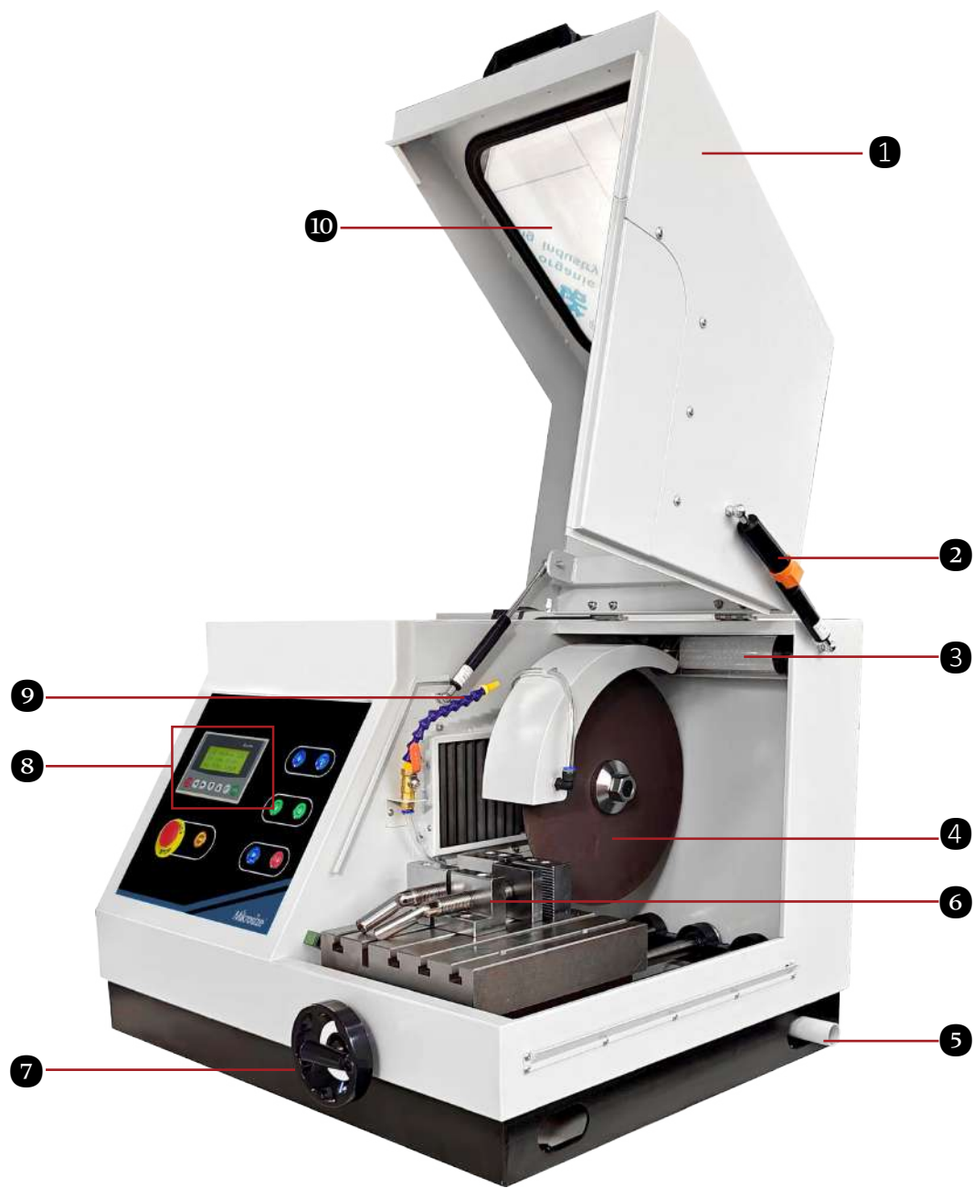
1. Protective housing 2. Support rod 3. Lighting lamp 4. Cut-off wheel 5. Outlet pipe port 6. Clamp 7. Handwheel 8. Screen and buttons 9. Coolant nozzle 10. Transparent observation window
