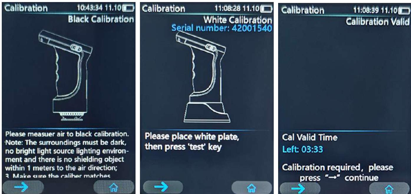
**The black-and-white calibration operation of the iColor-T407 spectrophotometer is simple and it is a crucial step for ensuring measurement accuracy.**
