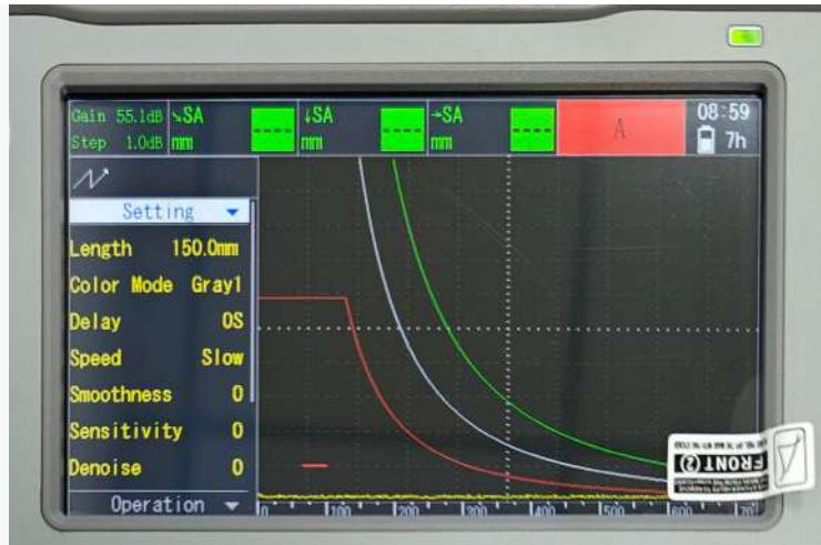
Only supports generating B-scan images in straight probe mode
