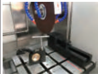
Cutting Chamber with Infrared Laser Positioning
